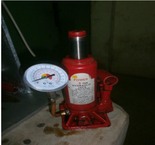
Fig. 4(e). Pressure Gauge connected to Hydraulic Jack
