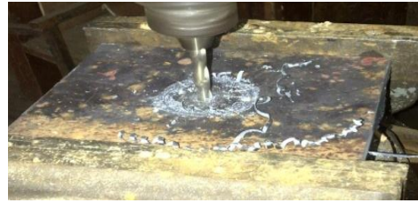
Fig. 4(b). Drilling the Top Plate
