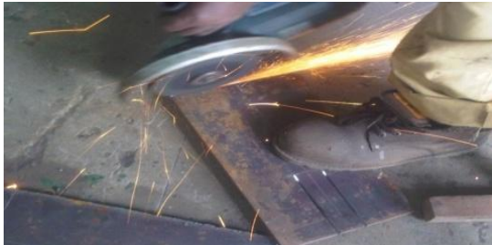
Fig. 4C. Cutting Side Frames for Casing
