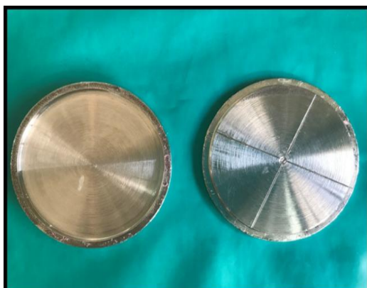
Fig. 1. Stainless Steel Die (ADA Specification no. 19)
