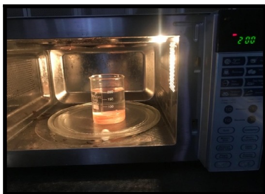
Fig. 4. Sample placed in microwave for 2 min at 430 W
