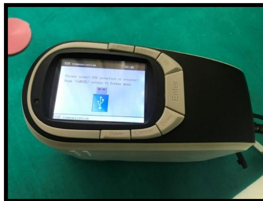
Fig. 5. Spectrophotometer Color Guide 45/0 used for Sample testing
