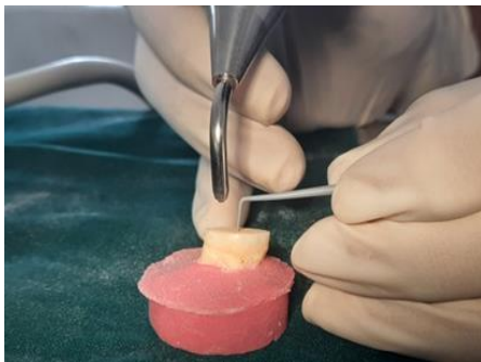
Fig. 5. Dentin pretreatment with aluminium oxide air abrasion
