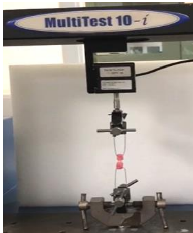
Fig. 13. Sample subjected to Microshear stress
