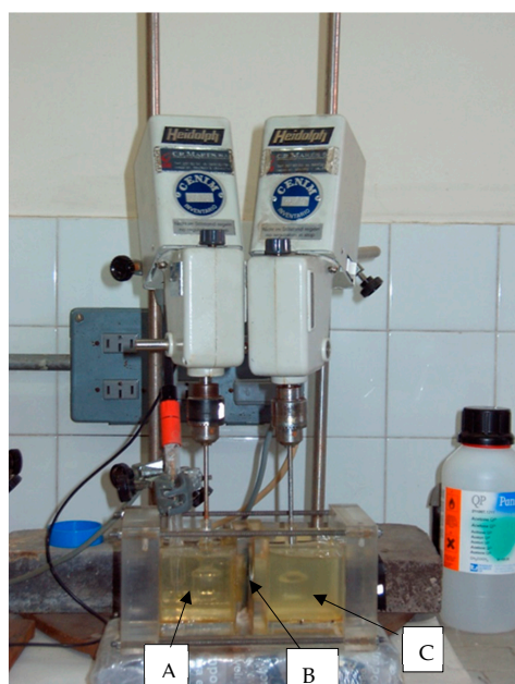
Figure 1. Permeation cell. A: feed phase; B: membrane support; and C: stripping phase.
