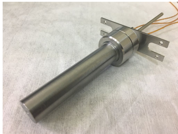
Figure 9. Novel coaxial–heater hollow cathode design with molybdenum cathode tube and keeper.
