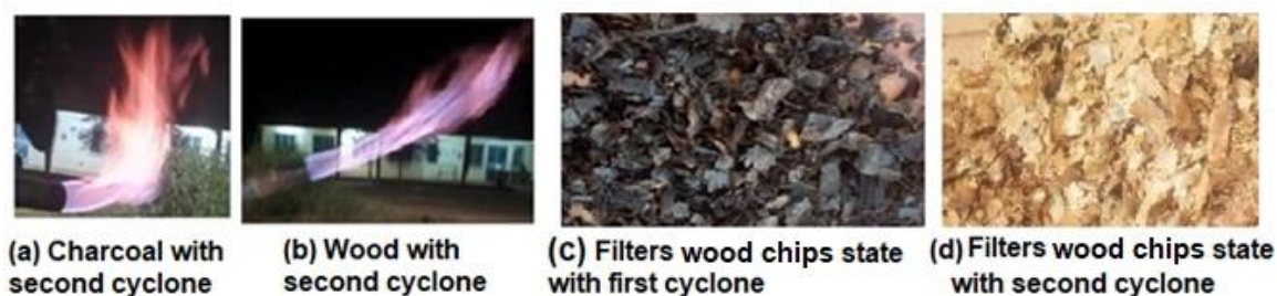
Fig. 11. Combustion flame quality with the second cyclone separator
