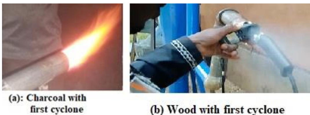
Fig. 9. Syngas combustion with first cyclone with charcoal and wood as combustible
