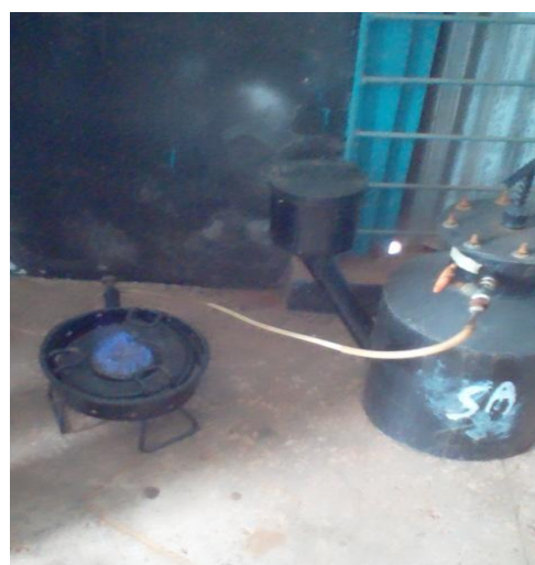
Fig. 3. Flammability check using a gas burner
