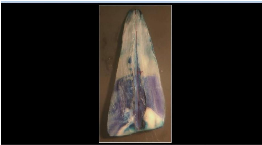
Fig. 8. Group-IV: Measurements of dye penetration in Ceraseal samples showing maximum and minimum values
