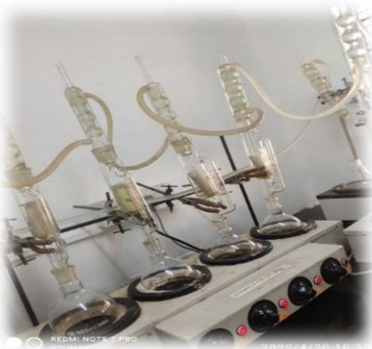
Fig. 1. Experimental set-up for extraction of rosemary essential oil by Hydro distillation
