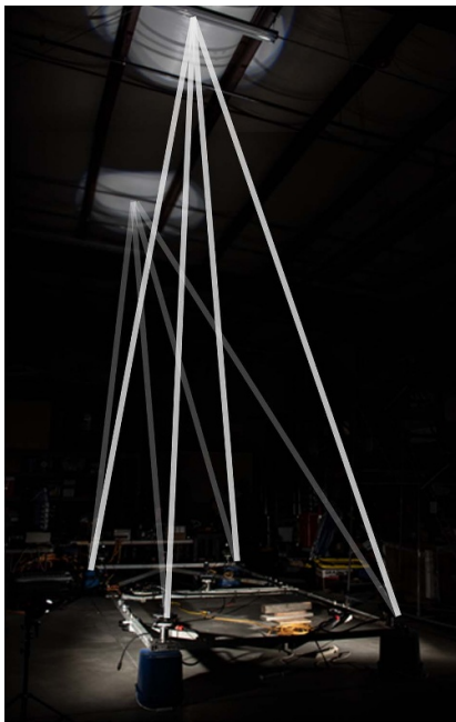
Figure 3. Attainment of two focal points at a solid boundary (target range = 8 m). Demonstrated via convergence of five spotlight beams, each with beam spread angle greater than that of s-ADP, mounted on the C-ADP's 5 actuation units. Image taken in two shots and overlaid, beam schematic superimposed. Conducted during laboratory commissioning and verification of control software.
