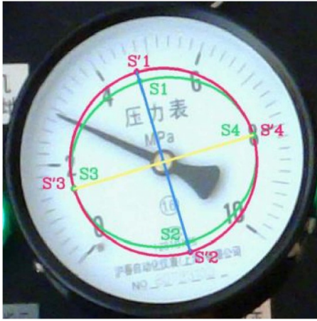
Figure 4. The result of the long and short axes of the ellipse where the scale value of the meter is located, and the intersection with the ellipse and the circle is also shown.
