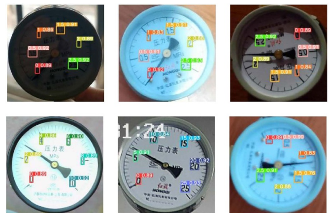
Figure 14. Meter image detection results in different environments.
