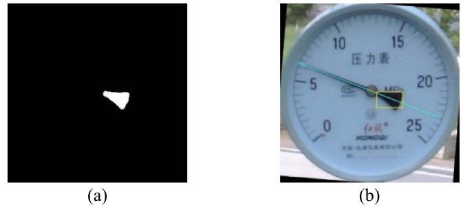
Figure 8. Interpretation diagram of fitting result of pointer linear equation. (a) Treatment results of pointer root. (b) Pointer straight line fitting and pointer root area frame fitting results.
