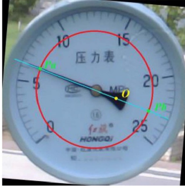
Figure 9. Explanation diagram of pointer direction solution.
