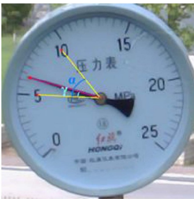
Figure 10. Interpretation diagram of the angle method.
