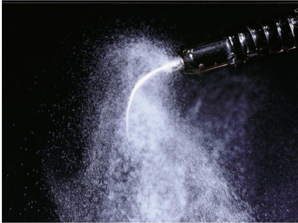
Fig. 3. The visible aerosol cloud produced by an ultrasonic scalar using a flow of 17 milliliters per minute of coolant water
