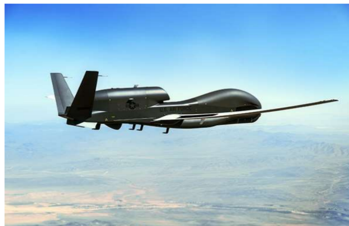
Figure 2. Example of a fixed-wing UAV: The Northrop Grumman RQ-4. Photo courtesy of Northrop Grumman [3].
