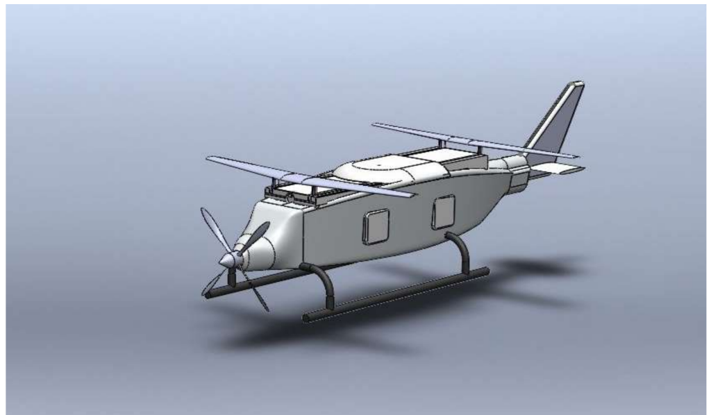
Figure 5. A snapshot of the animation of a SolidWorks conceptual design of an RA-driven VTOL aircraft.
