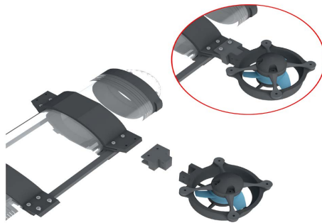
Figure 4. An adapter whose angle is 90 degrees helps thrusters to be mounted on the enclosure clamp.
