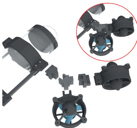
Figure 5. Adapters with 90-degree angles and splits are used for mounting purposes in the design part.
