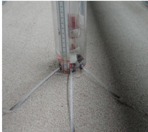
Fig. 1. Photo of a circular pier with a water jet injection on the pier surface
