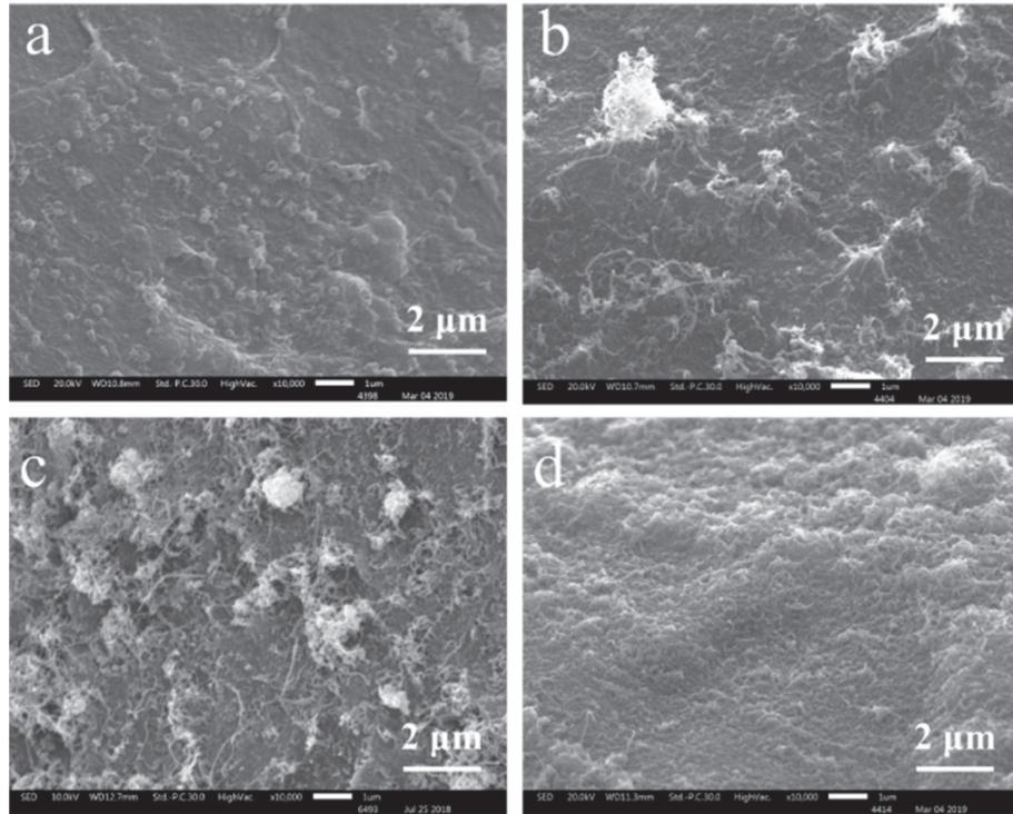
FIGURE 4: Surface morphology of mm-MWNTs-PDA@CaSA-Caps. MWNTs concentrations are (a)  $0.1 \text{ g}\cdot\text{L}^{-1}$ , (b)  $0.4 \text{ g}\cdot\text{L}^{-1}$ , (c)  $0.6 \text{ g}\cdot\text{L}^{-1}$ , and (d)  $1.0 \text{ g}\cdot\text{L}^{-1}$ .
