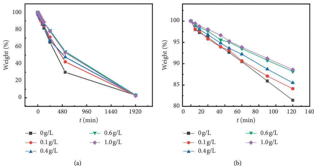
FIGURE 6: Effect of MWNTs concentration on water loss ratio of capsules at (a) test time 0–1920 min and (b) test time 0–120 min.
