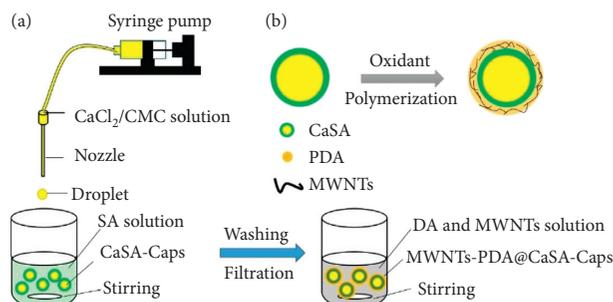
FIGURE 1: (a) Preparation of mm-MWNTs-PDA@CaSA-Caps. (b) Structure of mm-MWNTs-PDA@CaSA-Caps.
