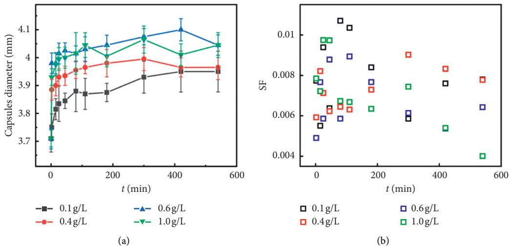
FIGURE 5: Effect of MWNTs concentration on (a) particle size and (b) SF of capsules during the reaction process.
