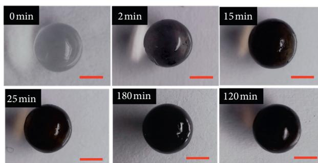
FIGURE 2: Images of mm-MWNTs-PDA@CaSA-Caps during the reaction process. Scale bar is 2 mm.
