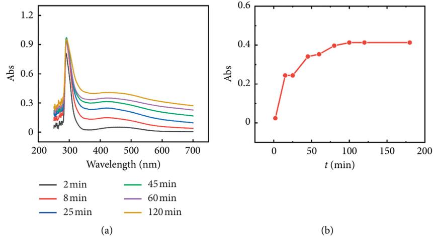
FIGURE 3: (a) The UV-vis spectra of DA solutions. (b) Absorption intensity in 350 nm during the reaction process.
